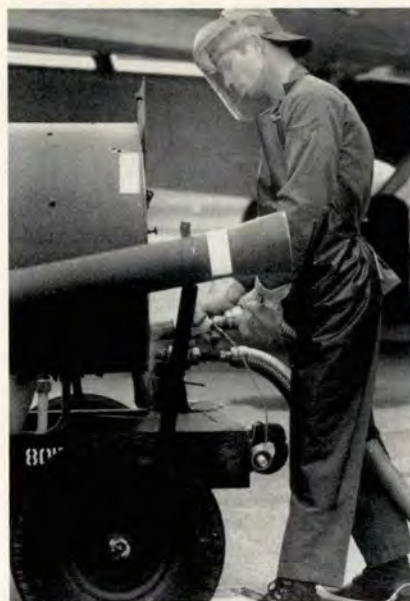
A fatigue cap must be worn when LOX servicing connectors are above eye level.
