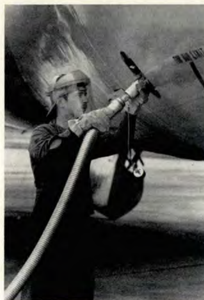
A fatigue cap must be worn when LOX servicing connectors are above eye level.
