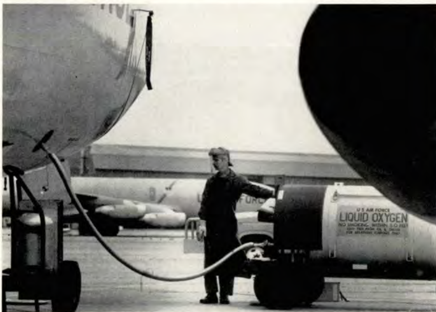
The LOX servicing unit should be located the maximum distance from the aircraft, and the hose should be free of kinks and sharp bends.
